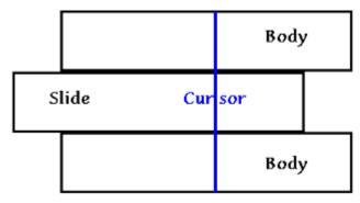
Scales appear on both the body and the slide, and on both sides of the rule. One side alone, or both sides together can be used in making a calculation.
